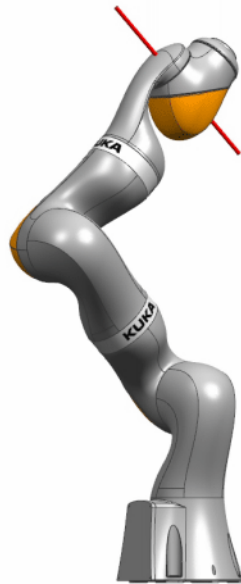
Fig. 15-26: A_5 = \pm 90^\circ (\pi/2) and A_6 = 0^\circ
