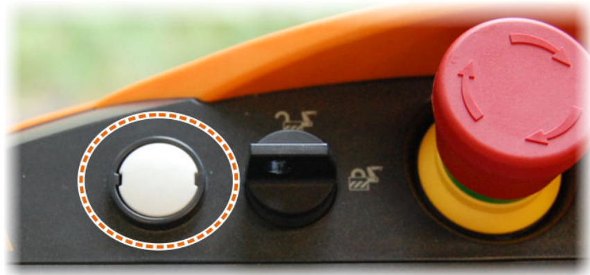
Fig. 6-5: Disconnecting the smartPAD button
